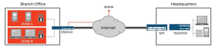
The SSG140 deployed at a branch office for secure Internet connectivity and site-to-site VPN to corporate headquarters. Internal branch office resources are protected with unique security policies for each security zone.
