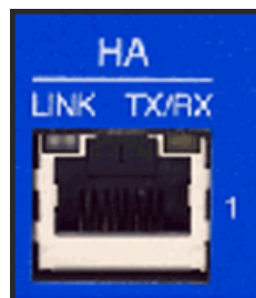
Figure 3: High Availability Interface Port LEDs
