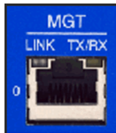
Figure 2: Management Interface Port LEDs
