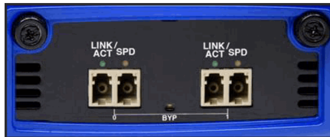
Figure 5: Fiber Port LEDs
